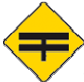
T-junction with dual carriageway
