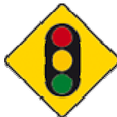
Traffic signals ahead
